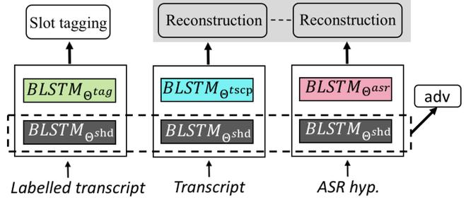
**Fig. 1.** Architecture of the proposed method which includes three tasks: transcript side slot-tagging, transcript side and ASR-hypotheses side reconstructions. The framework contains four BLSTM encoder for feature learning, one of which is shared by three tasks and the others are private for each task.
